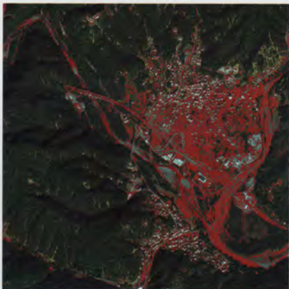
Figure 1 - Landslide and flooding map for Borghetto di Vara, Italy, where the impact of the high intensity storm of the October 25 th , 2011, was most severe. The area suffered massive flooding and widespread mass movements. Mapping obtained by processing very high spatial resolution satellite images taken on October 28 th , 2011.
