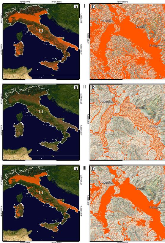
**Fig. 7.** Maps showing zonation of non-susceptible landslide areas in Italy. Red colour shows non-susceptible areas, and other colours show terrain outside non-susceptible landslide areas. (Ia) Map prepared adopting method I, Eq. (6). (IIa) Map prepared adopting method II, Eq. (7). (IIIa) Map prepared adopting method II, Eq. (8). Insets (Ib, IIb, IIIb) show enlargements for a portion of study area in Umbria, central Italy. See text for explanation. Background images of insets: ©2013 Google.
