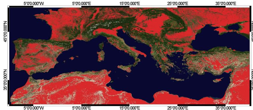
**Fig. 9.** Map showing zonation of non-susceptible landslide for the landmasses surrounding the Mediterranean Sea. Red shows non-susceptible areas, and other colours show terrain outside non-susceptible areas. Zonation was obtained using the QNL model, Eq. (8). See text for explanation.
