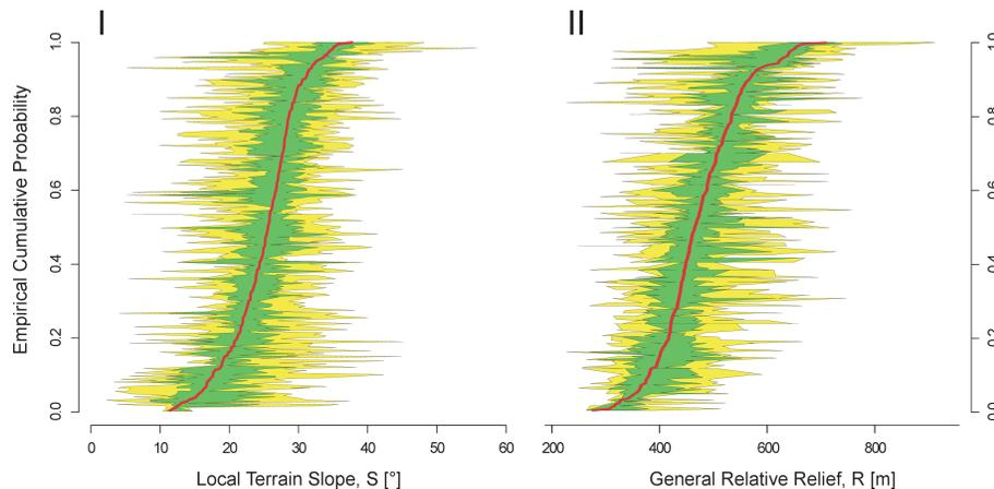
**Fig. 4.** Empirical Cumulative Distribution Function (ECDF) of (I) local terrain slope  $S$  and (II) regional relative relief  $R$  computed for each landslide shown in the Valcamonica inventory map,  $L$  in Table 1 (Antonini et al., 2000). Red line shows ECDF for the median (50th percentile), green area shows 25th–75th percentile range, yellow area shows 5th–95th percentile range.
