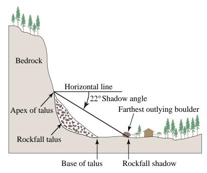
**Figure 4.** Sketch of rockfall talus at base of slope and outlying boulders illustrating the limit of the rockfall shadow angle (Wieczorek and others, 1999).
