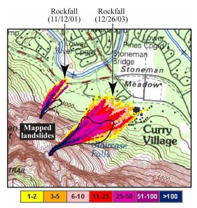
**Figure 5.** Comparison between the mapped landslides (thick black lines) and the simulated rockfalls for the November 12, 2001, event (left) and the December 26, 2003, event (right). Colors show the number of rockfall trajectories.
