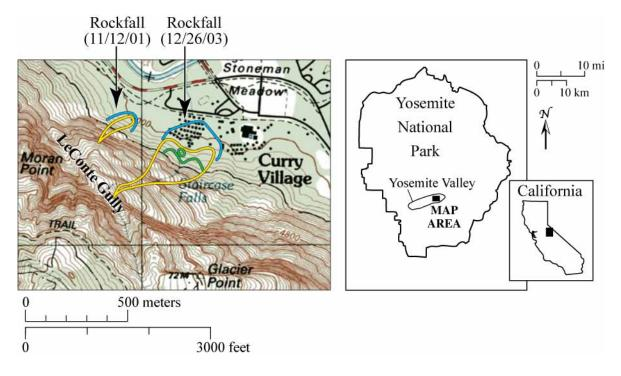
**Figure 1.** Topographic map of Glacier Point-Curry Village in Yosemite Valley, California, with two rockfalls from Staircase Falls into Curry Village. Yellow lines show the initial release, travel track, and continuous rock debris deposit region. The green line depicts where trees were knocked down, and the blue lines show the limit of flyrock.
