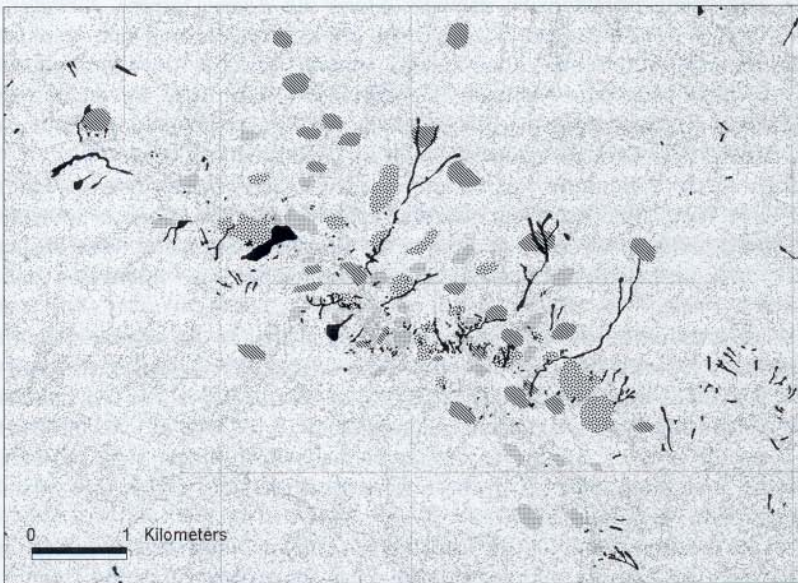
Figure 4. Armea valley, Imperia Province. The map shows landslides triggered by the high intensity rainfall event of 23-24 November 2000 (in black), and the areas where landslides produced by the 8-11 December 1910 event were reported. For the latter, different patterns represent different landslide abundance: light dotted pattern = few (1-2) landslides; oblique pattern = many (3-10) landslides; coarse dotted pattern = very many (> 10) landslides.
