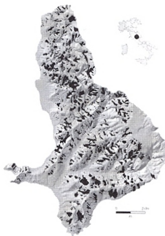
Fig. 1 Multi-temporal landslide inventory map for the Collazzone area
