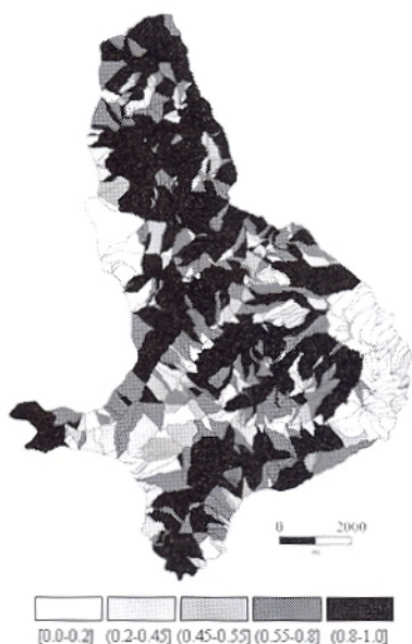
Fig. 2 Map showing spatial probability of landslide occurrence (landslide susceptibility) in five classes, obtained through discriminant analysis of 46 thematic variables. Square bracket indicates class limit is included, round bracket indicates class limit is not included
